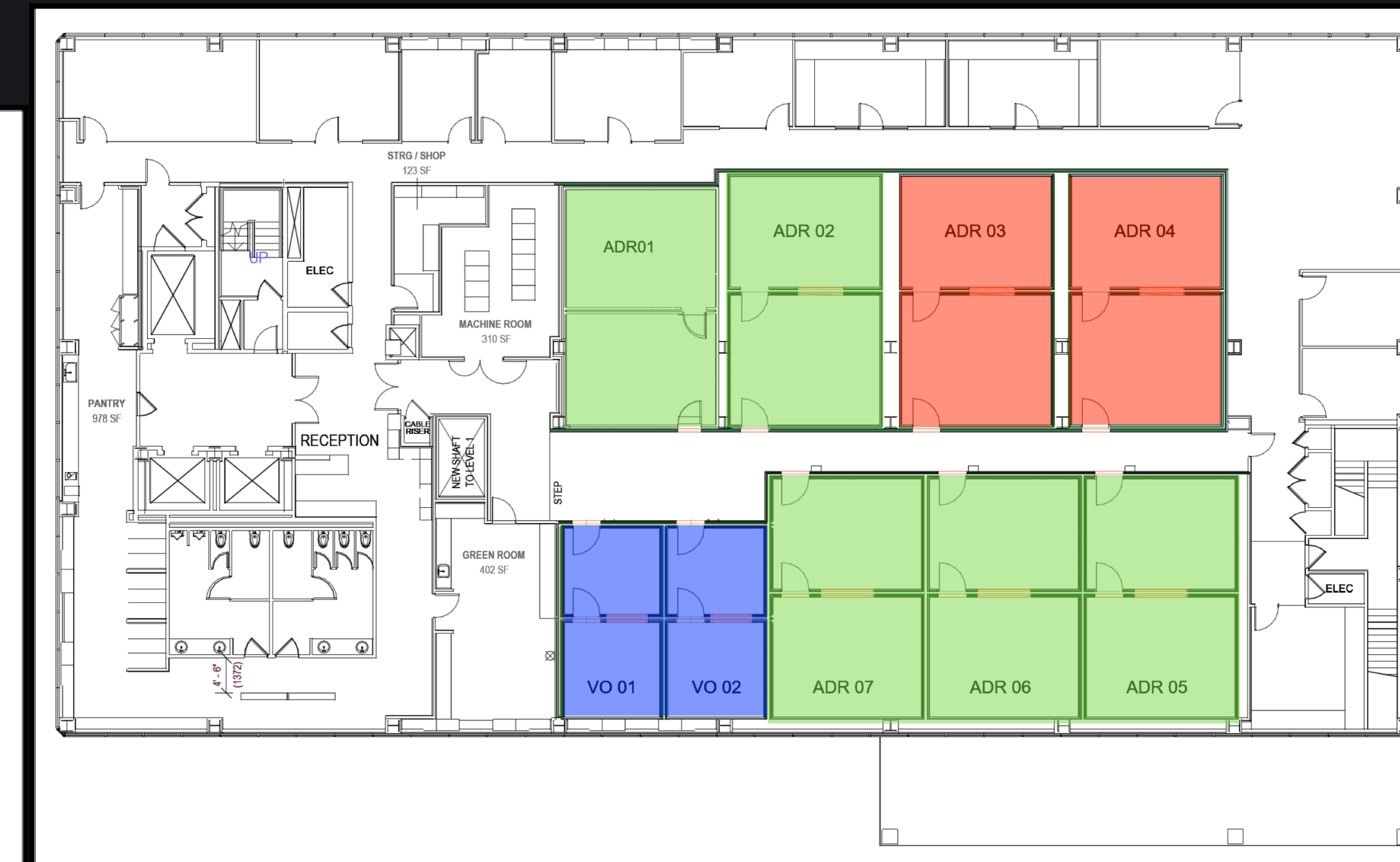
Ground 2: four ADR rooms, two hybrid ADR with 5.1 control, two VO booths.
